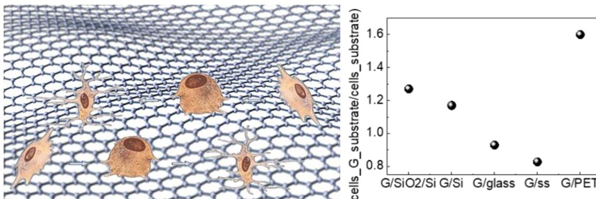
**Figure 1:** (left) Sketch of osteoblastic cells on graphene. (right) Ratio between the number of cells attached on graphene on SiO<sub>2</sub>/Si, Si, glass, stainless steel (SS) and plastic substrates and the number of cells attached on the corresponding substrates, after 2 days.
