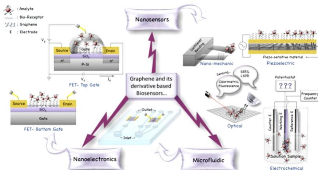
**Figure 1:** Schematic illustration of the sensing tactics involved in a graphene-based biosensor for in vitro and in vivo applications [from: N. Chauhan et al. J. Mat. Res. 32, 2860 (2017)]
